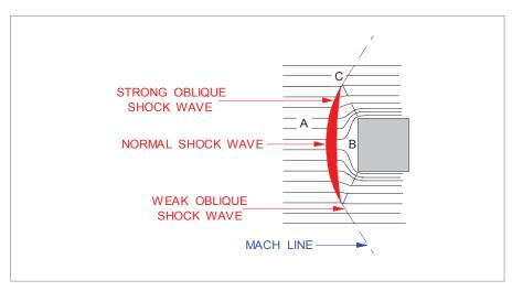
Figure 13.10 Normal & oblique shock waves
