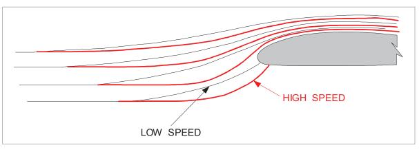
Figure 13.12 Streamlines at low & high subsonic speeds
