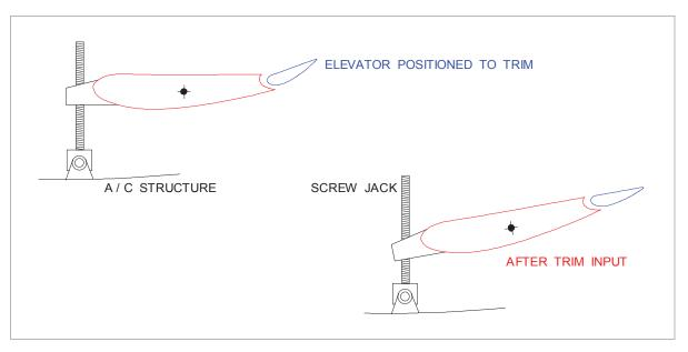
Figure 11.26 Variable incidence (trimming) tailplane
