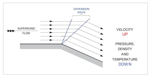
Figure 13.40 Supersonic flow at a convex corner with expansion wave
