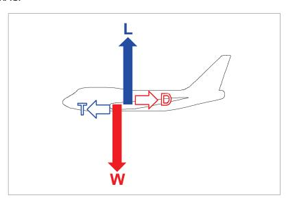
Figure 1.5 The forces of weight, lift, thrust & drag
