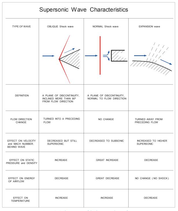
Figure 13.42 Characteristics of the three principle wave forms
