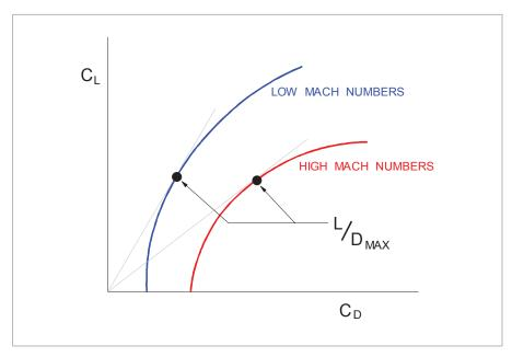
Figure 13.17 Effects of Mach number on  $C_{\rm L}/C_{\rm D}$  polar
