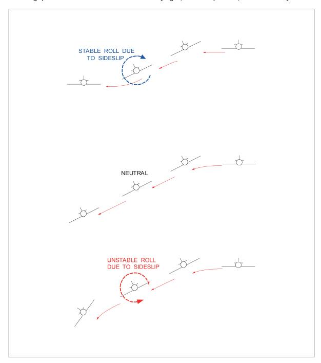
Figure 10.68 Static lateral stability
