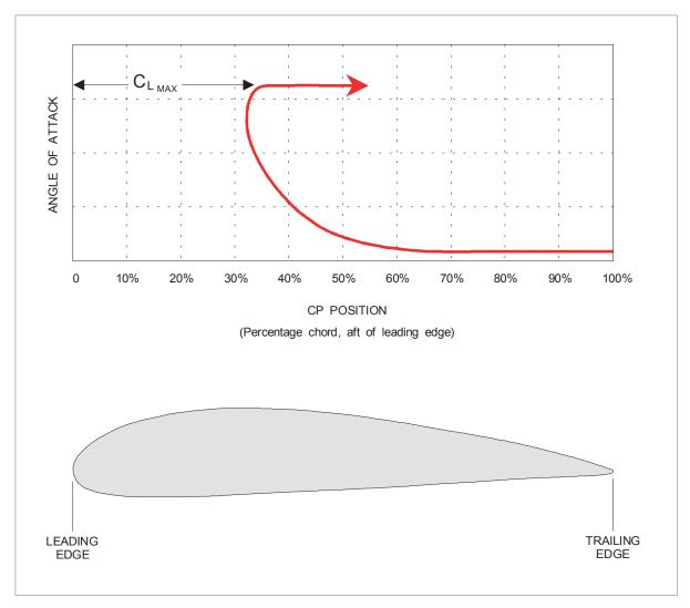
Figure 4.9 CP movement with angle of attack
