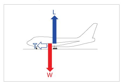
Figure 1.4 The forces of weight, lift & thrust
