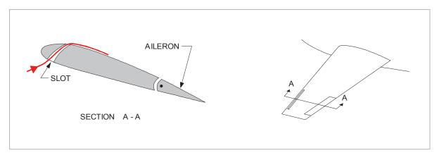
Figure 7.11 Leading edge slot
