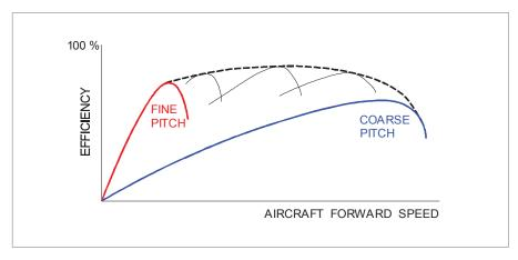
Figure 16.10 Efficiency improved by varying blade angle
