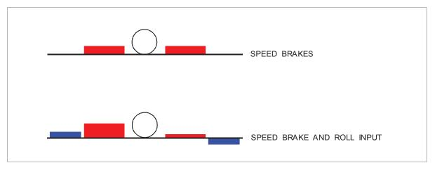
Figure 11.22 Mixed speed brake & roll input
