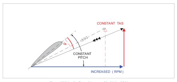
Figure 16.6 Angle of attack increased by higher RPM
