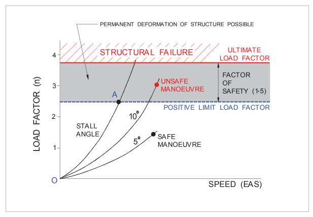
Figure 14.2 Loads imposed during manoeuvres
