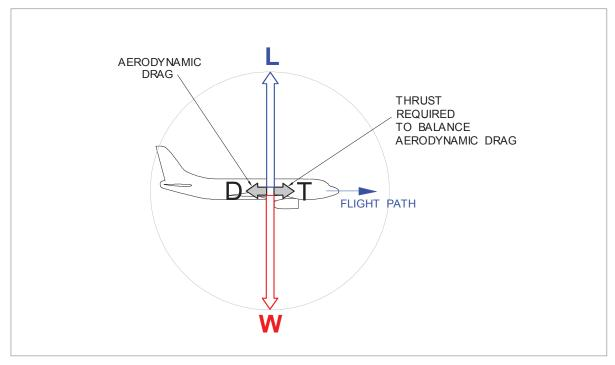
Figure 12.1 Forces in level flight
