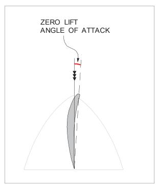
By turning the blades to their zero lift angle of attack, no propeller torque is generated and the propeller will stop, reducing drag to a minimum, as shown in *Figure 16.16*. This will improve climb performance because the ability to climb is dependent on excess thrust after balancing aerodynamic drag.
