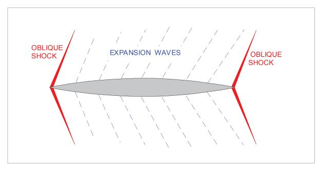
Figure 13.41 Expansion waves in a supersonic flow
