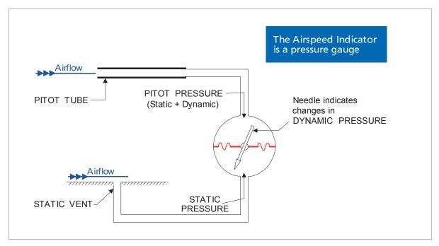
Figure 2.1 Schematic of the airspeed indicator (ASI)
