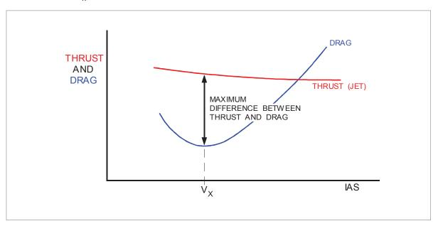
Figure 12.6 Variation of excess thrust with speed (JET)
