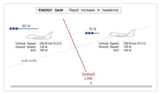
Figure 15.3 "Energy gain" due to increase in headwind
