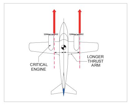
Figure 12.23 Critical engine
