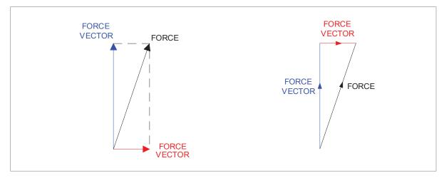
Figure 7.21 The resolution of a force into two vectors and the addition of vectors to form a resultant
