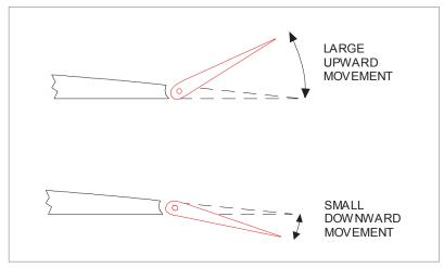
Figure 11.17 Differential ailerons
