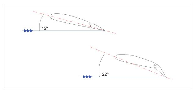
Figure 14.15 Low speed aileron reversal
