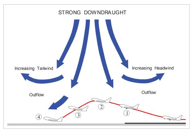
Figure 15.1 A microburst encounter during take-off
