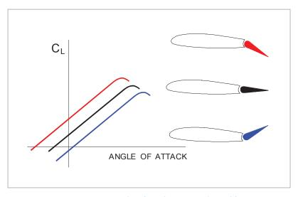
Figure 11.1 Control surface changes camber & lift
