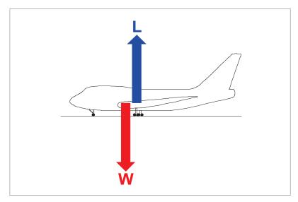
Figure 1.3 The forces of weight & lift
