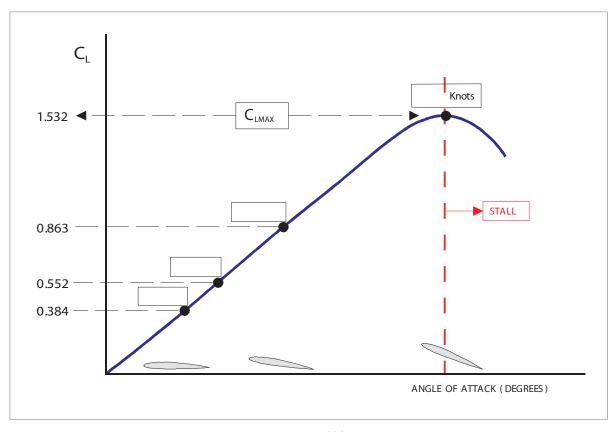
Figure 5.4 Typical lift curve
