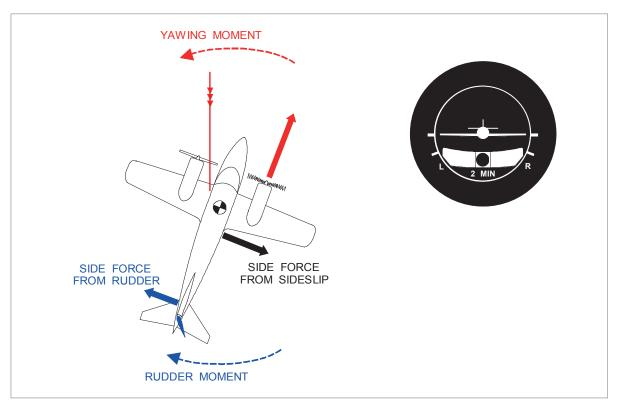
Figure 12.24 Wings level method
