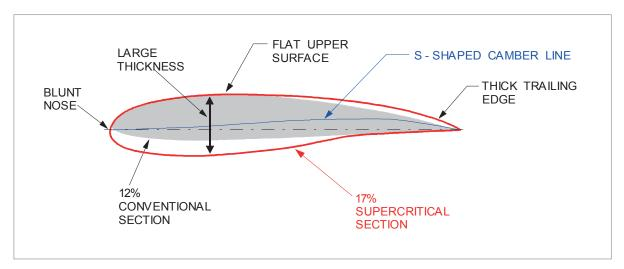
Figure 13.34 Supercritical aerofoil shape
