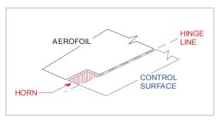
Figure 11.6 Horn balance
