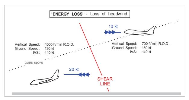
Figure 15.5 "Energy loss" due to loss of headwind
