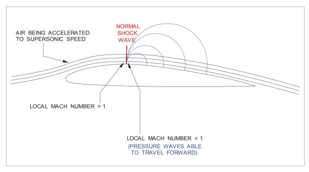
Figure 13.5 Shock wave at subsonic free stream Mach number
