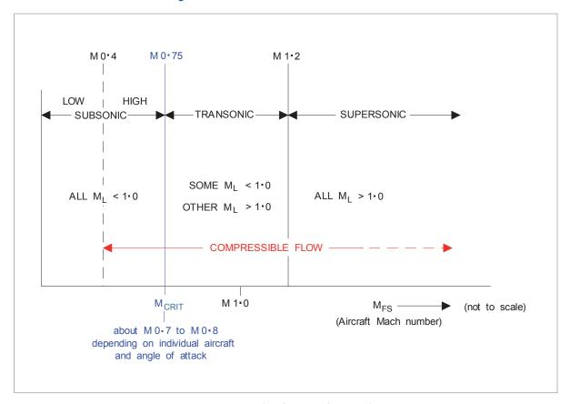
Figure 13.2 Classification of airspeed
