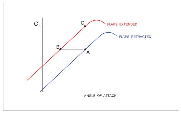
Figure 8.22 Deployment of flaps for landing
