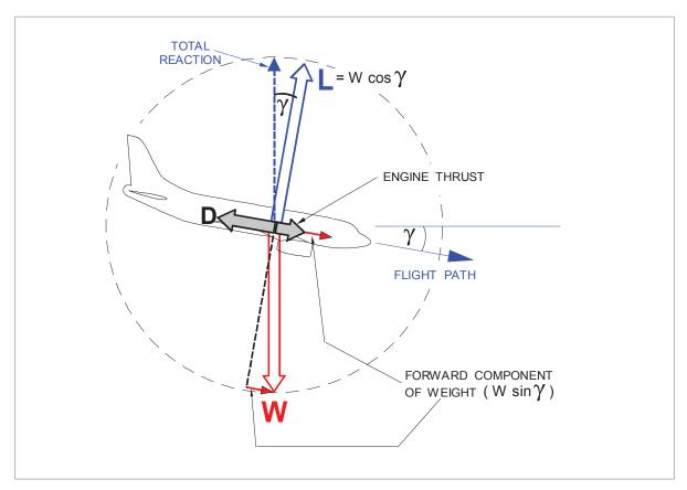
Figure 12.7 Forces in a power-on descent
