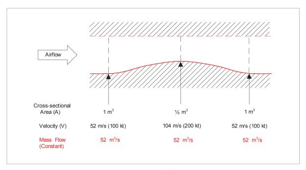
Figure 3.1 The principle of continuity
