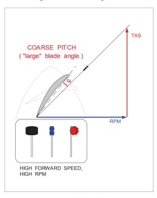
Figure 16.13 High TAS, high RPM
