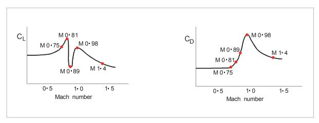
Figure 13.7 Changes in lift & drag in the transonic region
