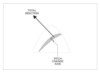
Figure 16.9 Aerodynamic twisting moment (ATM)
