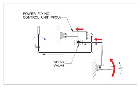
Figure 11.12 Power assisted flying control
