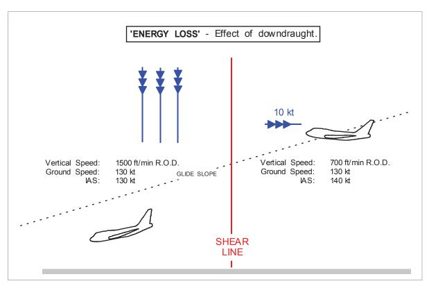
Figure 15.4 "Energy loss" due to downdraught
