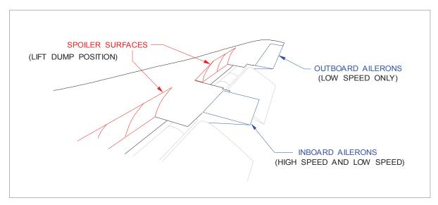
Figure 11.19 Inboard & outboard ailerons & spoiler surfaces
