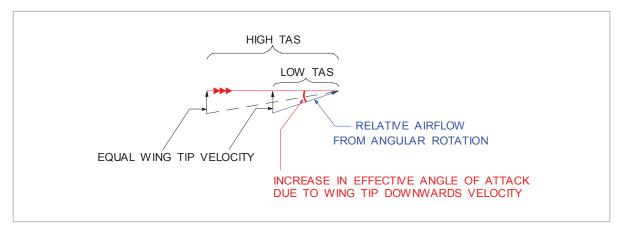
Figure 11.16 Aerodynamic damping in roll
