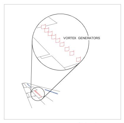
Figure 13.30 Vortex generators (blade type)
