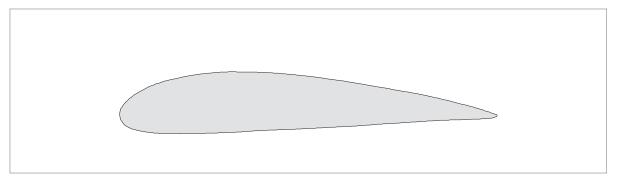
Figure 3.3 Typical aerofoil section
