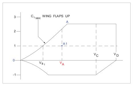
Figure 14.3 Design manoeuvring speed V
