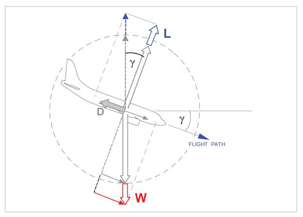
Figure 12.9 Increased weight: no effect on glide range
