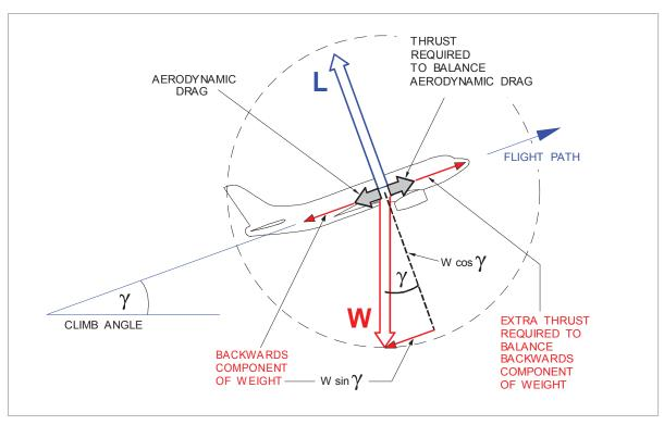
Figure 12.5 Forces in a steady climb
