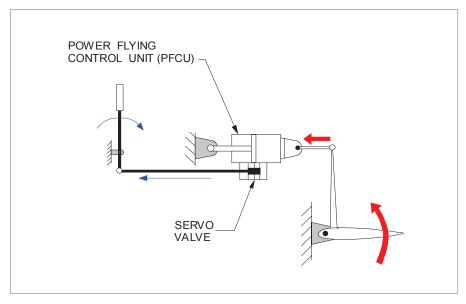
Figure 11.13 Fully powered flying control
