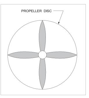
Figure 16.18 Solidity of a propeller
