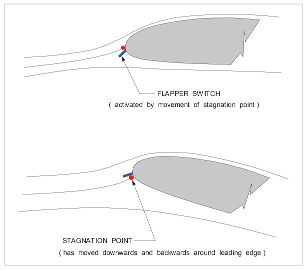
Figure 7.6 Flapper switch
