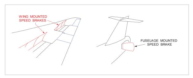
Figure 11.21 Wing mounted & fuselage mounted speed brakes
