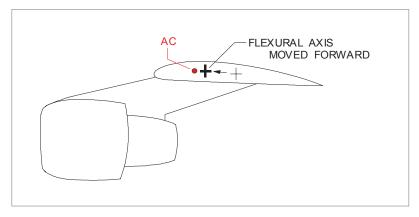
Figure 14.13 Wing mass balanced by podded engines
