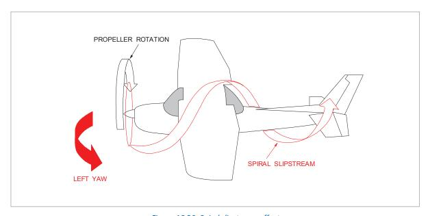
Figure 16.20 Spiral slipstream effect
