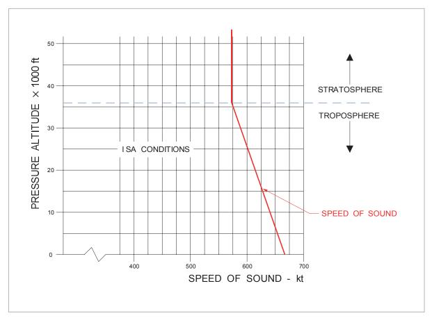
Figure 13.1 Variation of speed of sound with altitude
