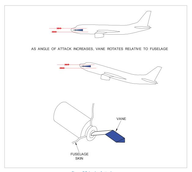
Figure 7.7 Angle of attack vane
