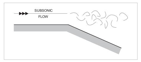
Figure 13.39 Subsonic flow at a convex corner
