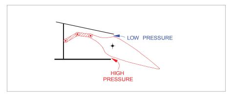
Figure 11.7 Internal balance
