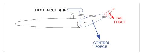
Figure 11.9 Anti-balance tab
