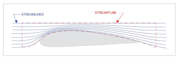
Figure 3.4 Streamlines & a streamtube
