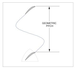
Figure 16.2 Geometric pitch
