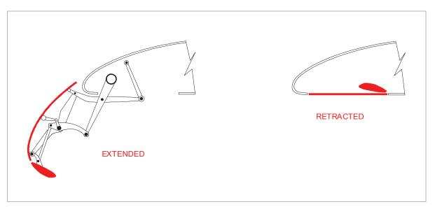
Figure 8.12 Variable camber leading edge flap
