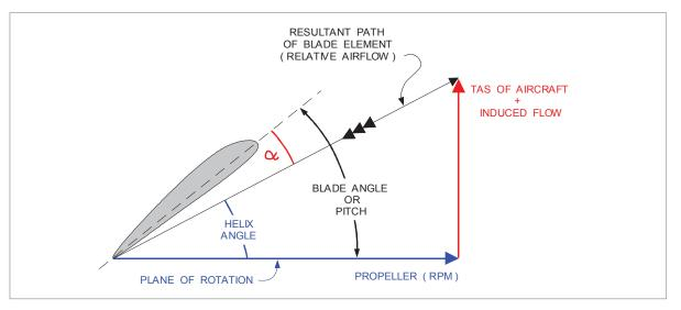
Figure 16.4 Angle of attack
