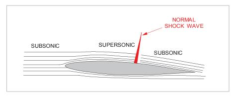
Figure 13.9 Normal shock wave formation
