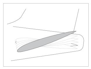
Changing the incidence of an aerofoil will change its lift. The usual application of this system is for pitch control - the all moving (slab) tailplane. There is no elevator; when the pilot makes a pitch input, the incidence of the whole tailplane changes.
