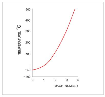
Figure 13.35 Surface temperature rise with Mach number
