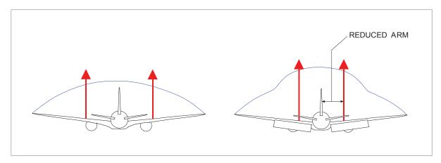
Figure 10.75 Partial span flaps reduce lateral stability
