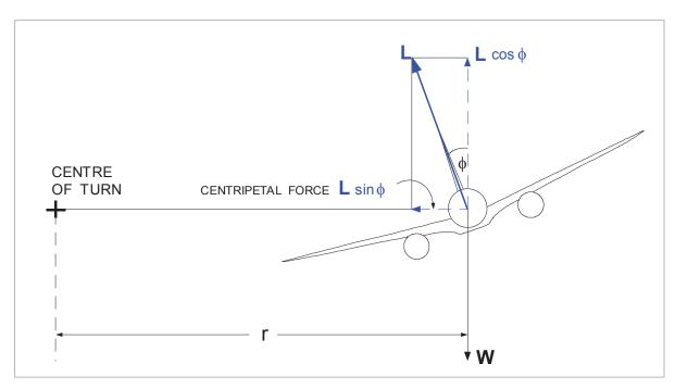
Figure 12.14 Forces acting in a steady turn
