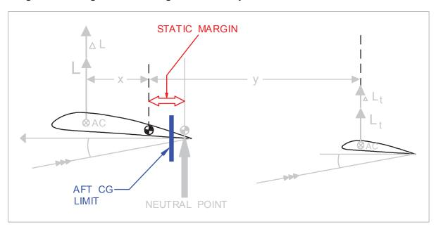
Figure 10.10 Static margin & aft CG limit
