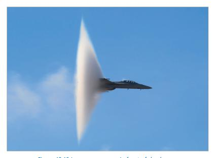
Figure 13.19 Low pressure area in front of shock wave
