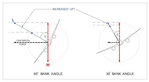
Figure 12.16 Increased lift required in a turn
