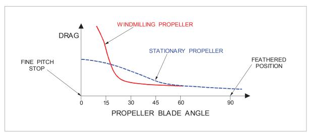
Figure 12.26 Propeller drag
