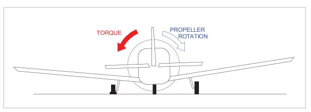
Figure 16.19 Torque reaction giving left turn during take-off
