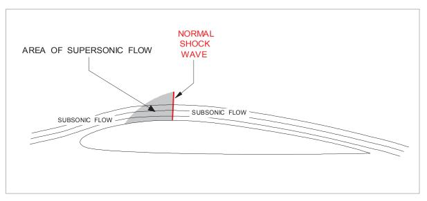
Figure 13.6 Mixed supersonic & subsonic airflow at transonic speeds
