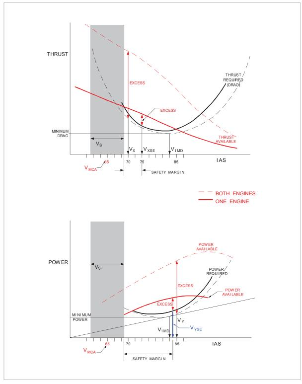
Figure 12.28 Excess thrust & excess power.
