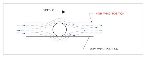
Figure 10.70 Wing - fuselage interference effect
