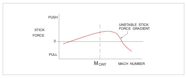
Figure 13.20 Reduction in stick force with increasing Mach number
