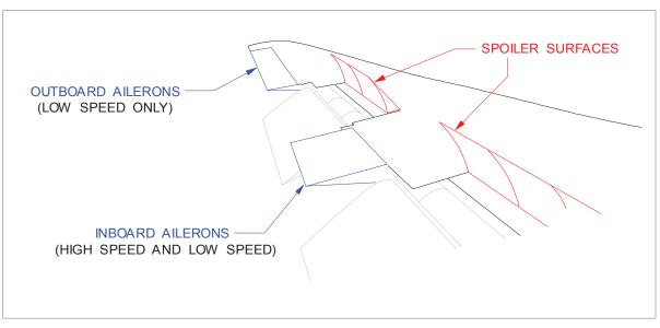
Figure 14.17 Inboard & outboard ailerons & roll spoilers
