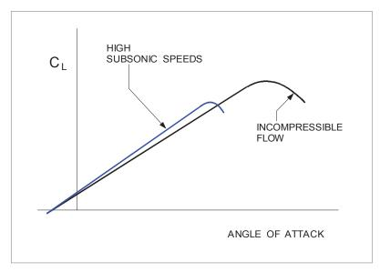
Figure 13.14 Effects of Mach number on lift curve
