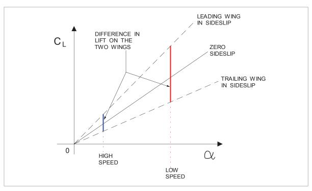
Figure 10.72 Effect of speed on 'Dihedral Effect' of swept wing
