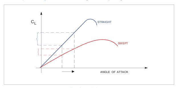
Figure 13.29 Effect of sweepback on sensitivity to gusts
