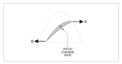
Figure 16.8 Centrifugal turning moment (CTM)
