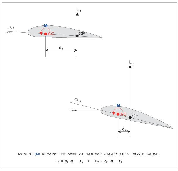
Figure 10.5 Aerodynamic centre (AC)
