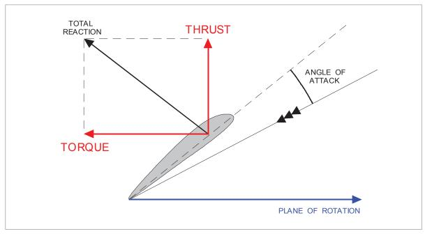
Figure 16.7 Thrust & torque
