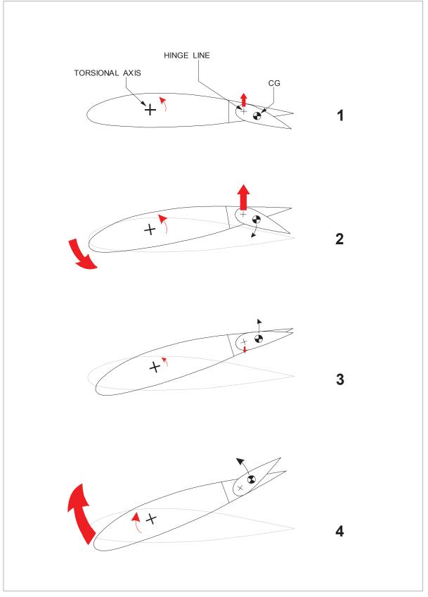
Figure 14.14 Torsional aileron flutter
