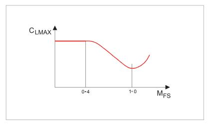
Figure 13.15 Effect of Mach number on C<sub>LMAX</sub>
