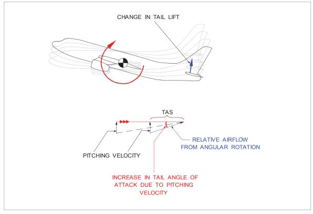
Figure 10.37 Aerodynamic damping
