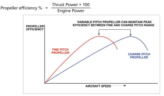
Figure 12.7 Propeller efficiency curves
