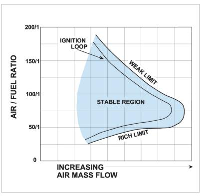
Figure 16.7 A typical combustion stability loop.
