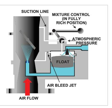
Figure 8.8 An air bleed mixture control.
