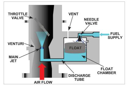
This carburettor employs two basic principles, those of the 'U' tube and the Venturi.
