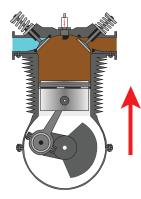
4. The exhaust valve is now open to atmosphere. The piston moving up forces the exhaust gas past it to the atmosphere. The atmosphere provides a resistance to the flow of exhaust gas which is termed 'EXHAUST BACK PRESSURE'. Because of this the pressure in the cylinder increases slightly which causes the temperature to rise also.
