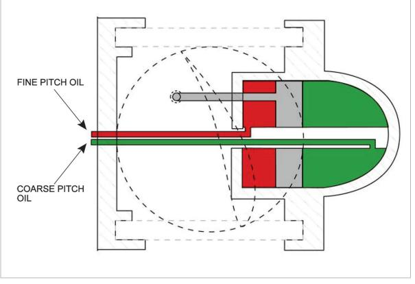
Figure 12.10 The double acting propeller.
