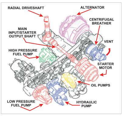
Figure 22.4 An external gearbox showing various accessories.
