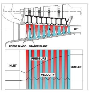
Figure 15.2 The changes in pressure & velocity through an axial flow compressor.
