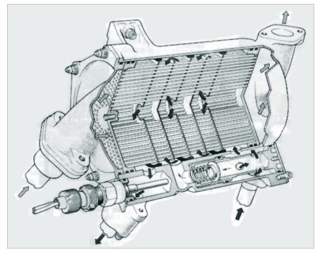
Figure 19.6 A fuel-cooled oil cooler
