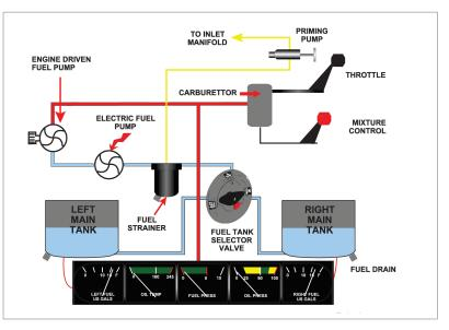
Figure 8.12 Single-engine light aircraft fuel system & engine priming system.
