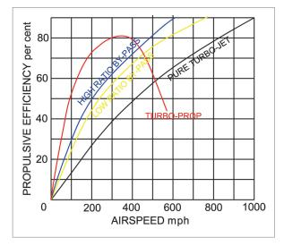
Figure 13.12 The propulsive efficiencies of gas turbine engines.
