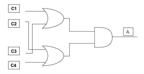
To get logic 1 output at A there must be a logic 1 input at:
