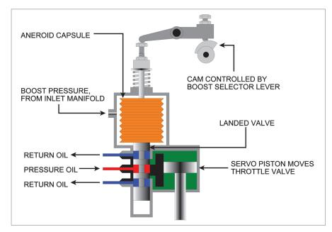
Figure 11.11 An automatic boost control unit.
