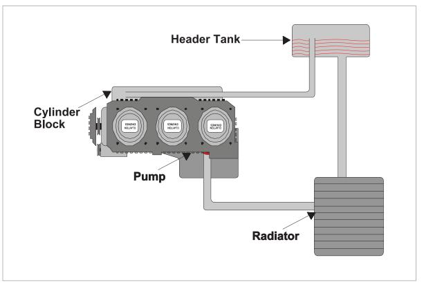
Figure 4.1 Liquid cooling system.
