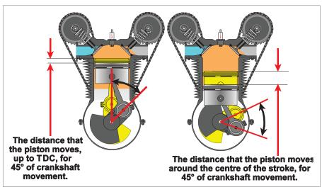
Figure 2.6 Ineffective crank angle
