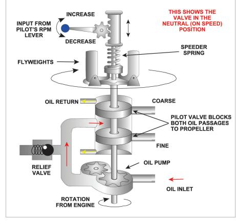
Figure 12.12 A simple constant speed unit.
