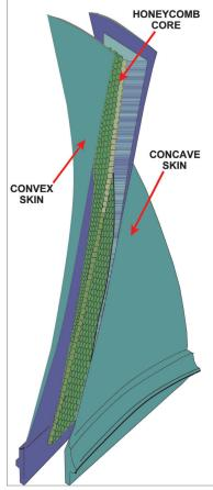
Figure 15.10 Wide chord fan blade construction.
