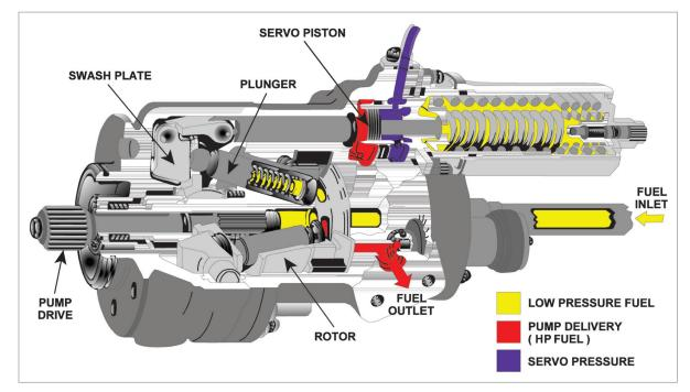
Figure 26.2 Axial piston type fuel pump (based on an original Rolls Royce drawing)
