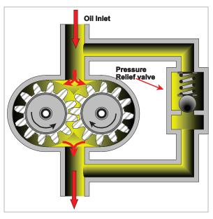
Figure 3.2 Spur gear pump
