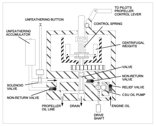
Figure 12.17 CSU with unfeathering accumulator
