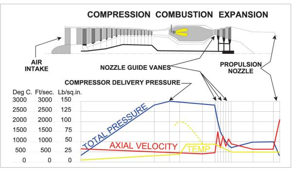
Figure 13.5 Changes in pressure, temperature & velocity in a single spool axial flow engine.
