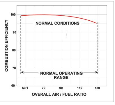
Figure 16.9 Combustion Efficiency and Air/Fuel Ratio.
