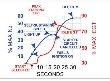
Figure 24.6 RPM/EGT starting relationship
