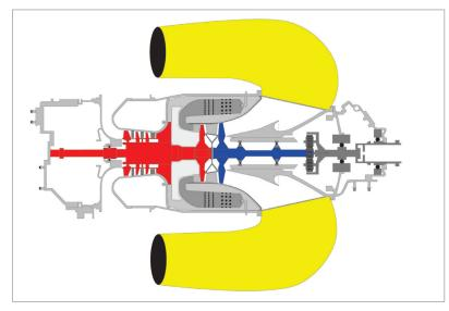
Figure 13.9 A single spool turboshaft engine incorporating a free power turbine.
