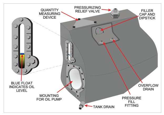
Figure 19.4 A typical oil tank.
