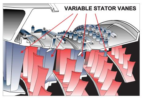
Figure 15.4 Typical variable stator vanes
