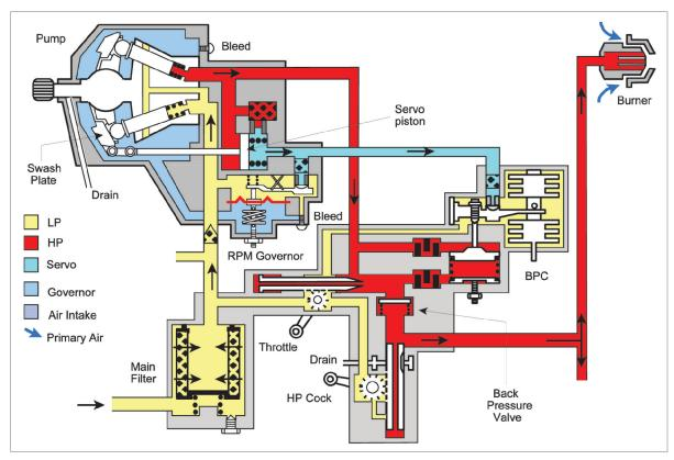
Figure 26.3 Hydro-mechanical fuel control
