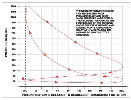
Figure 2.7 A typical indicator diagram
