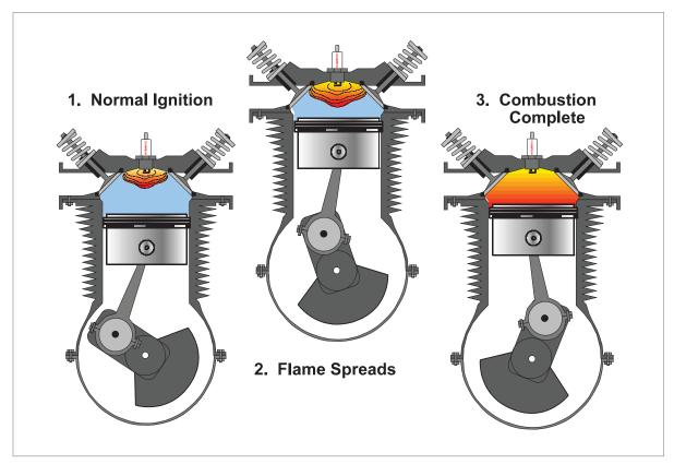
Figure 6.1 Normal combustion.
