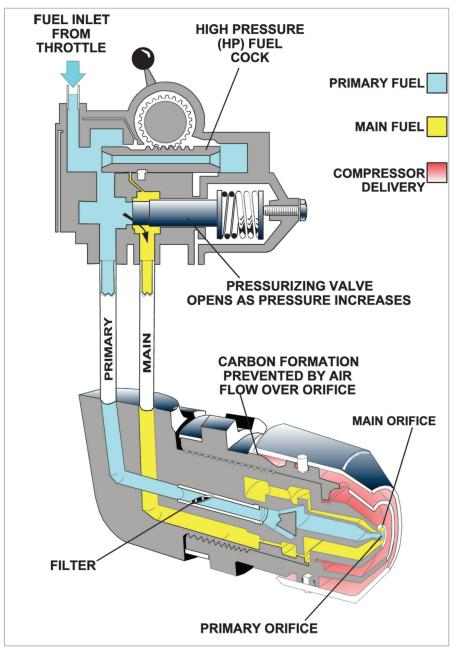
Figure 16.12 The duplex fuel spray nozzle.
