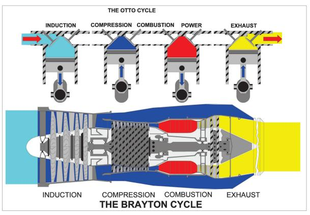
Figure 13.3 A comparison of the working cycles of the piston engine & the gas turbine engine.
