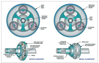
Figure 12.23 Spur & bevel planetary gears
