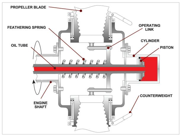
Figure 12.9 The single acting propeller
