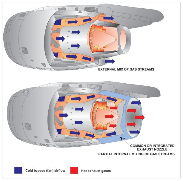
Figure 18.5 High ratio bypass engine exhaust systems.
