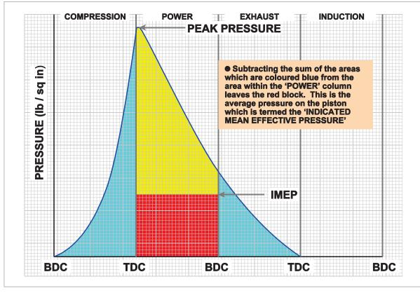
Figure 2.9 An indicator diagram plotted against stroke for simpler calculation of pressure areas
