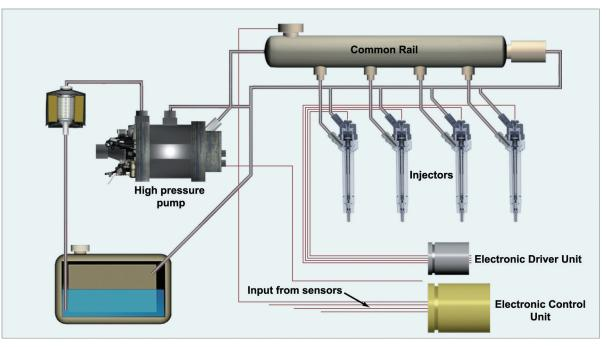
Figure 10.3 A common rail system.
