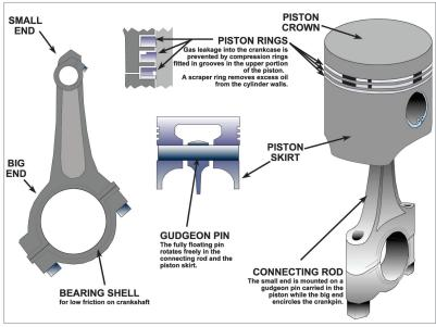
Figure 2.13 The piston and associated components
