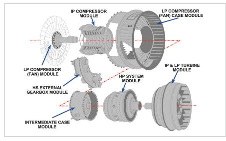
Figure 13.13 Modular construction units.
