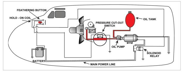
Figure 12.18 Typical feathering installation.
