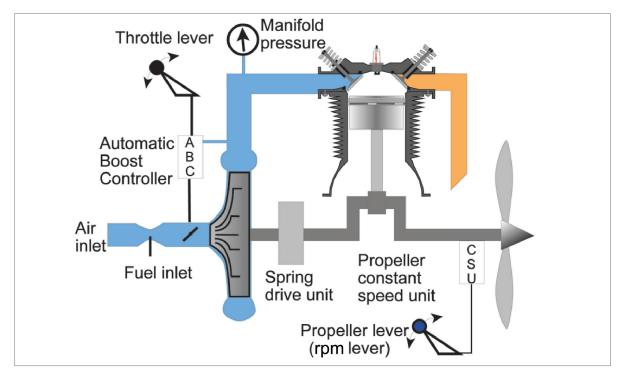
Figure 11.9 Internally driven supercharger - general arrangement.
