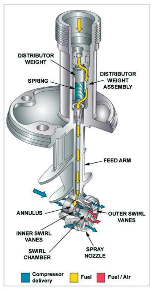
Figure 16.11 An airspray nozzle.
