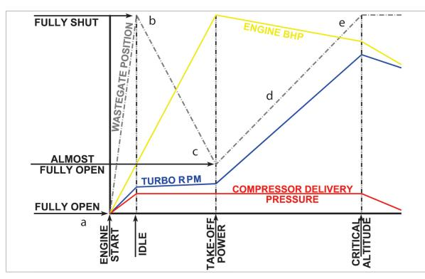
Figure 11.5 The relationship of wastegate position, engine power, manifold pressure & turbocharger rpm to each other.
