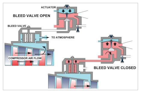
Figure 15.5 The operation of a compressor bleed valve.
