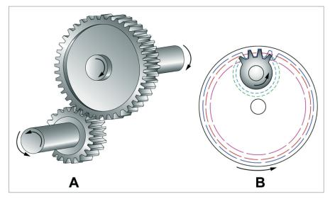
Figure 12.22 Two types of spur type reduction gear arrangement
