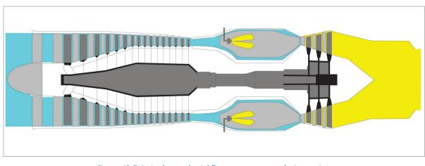
Figure 13.7 A single spool axial flow compressor turbojet engine.
