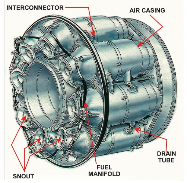
Figure 16.3 A multiple combustion chamber system.
