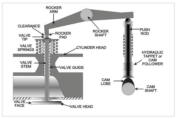
*Figure 2.15 Valve clearance*
