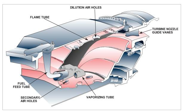
Figure 16.13 The vaporizing method of fuel feed.
