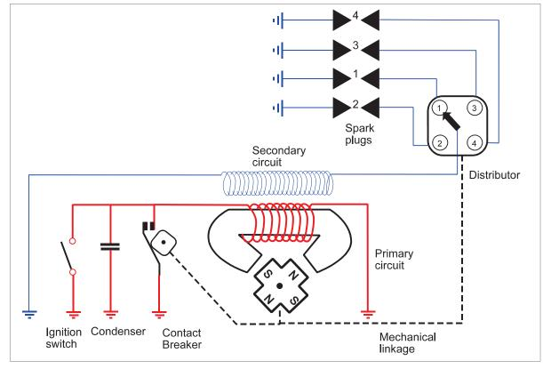
Figure 5.1 Magneto Circuit
