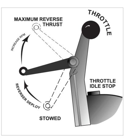
Figure 21.2 Throttle & reverse thrust lever.
