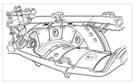
Figure 16.6 Details of annular combustion chamber (based on an original Rolls-Royce drawing).
