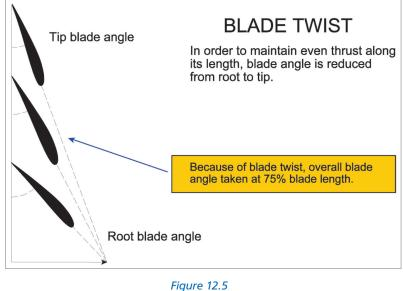
To even out the thrust developed along the blade, the angle of attack is maintained by reducing the blade angle from root to tip.
