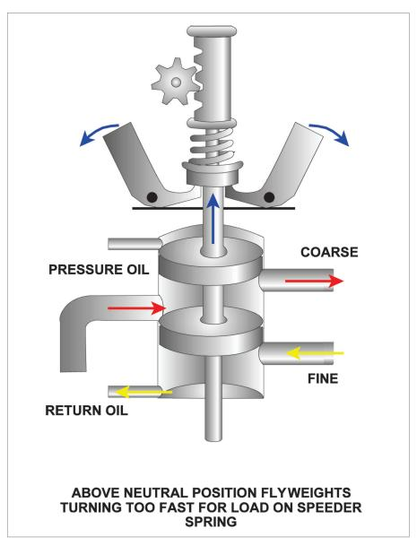
Figure 12.13 Overspeed condition.
