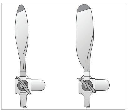
Figure 12.11 Propeller with various pitch angles.
