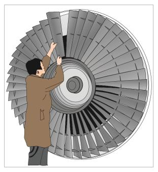
Figure 15.9 A high bypass ratio engine low pressure compressor or fan.
