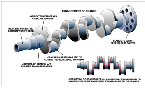
Figure 2.12 A four cylinder crankshaft
