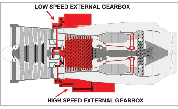
Figure 22.3 Spreading the load of accessories between two gearboxes.
