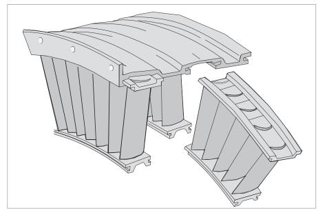
Figure 15.8 Segments of shrouded stator vanes.
