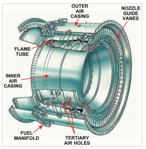
Figure 16.5 An annular combustion chamber.
