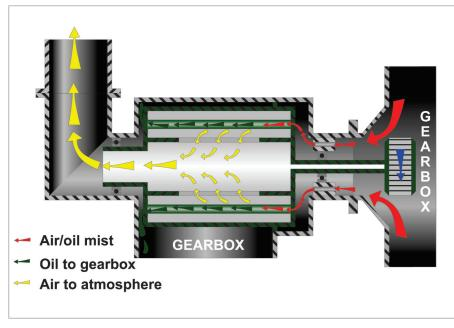
Figure 19.8 The centrifugal breather & vent.
