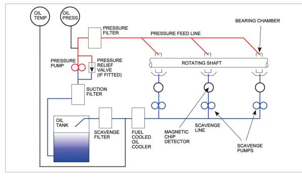
Figure 19.1 Schematic gas turbine oil system.
