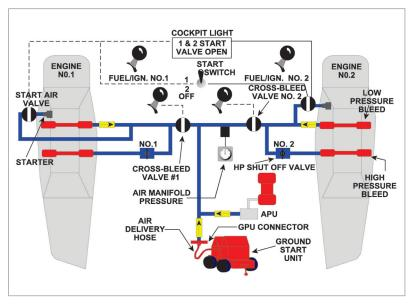
Figure 24.5 Two engine air starter layout
