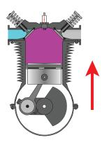
2. Both of the valves are closed trapping the induced mixture in the cylinder. The piston is moving up. The cylinder volume is decreasing. The cylinder pressure is increasing. The temperature of the charge is increasing. The mass of the charge is now fixed.
