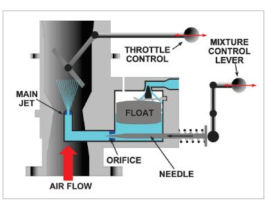
Figure 8.7 A needle type mixture control.
