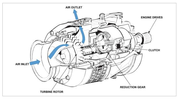
Figure 24.4 An air starter motor
