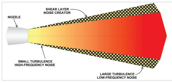
Figure 18.7 The pattern of noise created by jet exhaust.
