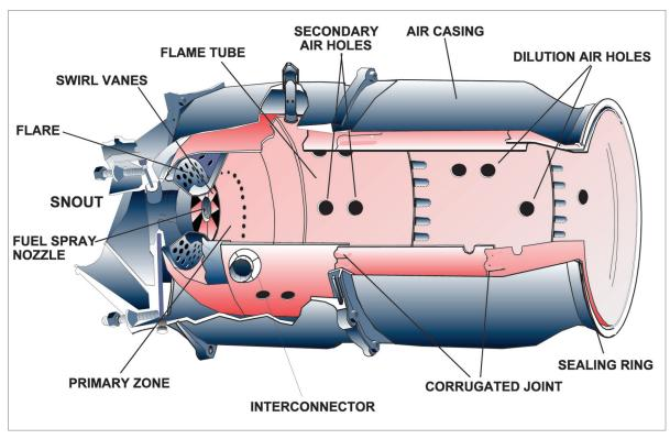
Figure 16.2 An early combustion chamber.
