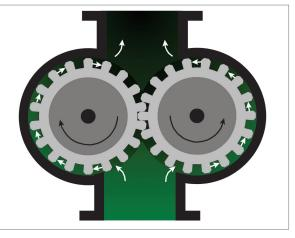
Figure 19.5 A gear type oil pump.
