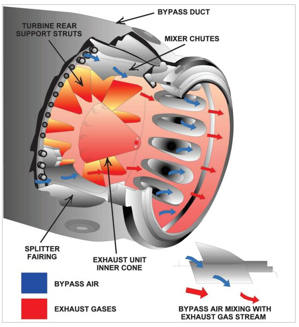
Figure 18.4 A low ratio bypass engine exhaust unit.
