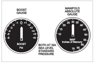
Figure 11.2 Manifold pressure indications.
