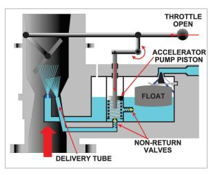
Figure 8.11 An accelerator pump.
