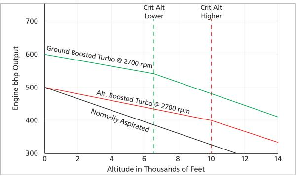
Figure 11.6 A comparison of the power curves of a normally aspirated engine & a turbocharged engine.
