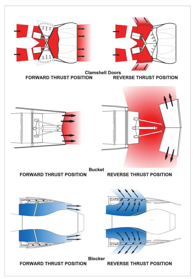
Figure 21.1 The types of reverse thrust systems.
