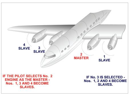
Figure 12.20 The master engine arrangement of a transport aircraft
