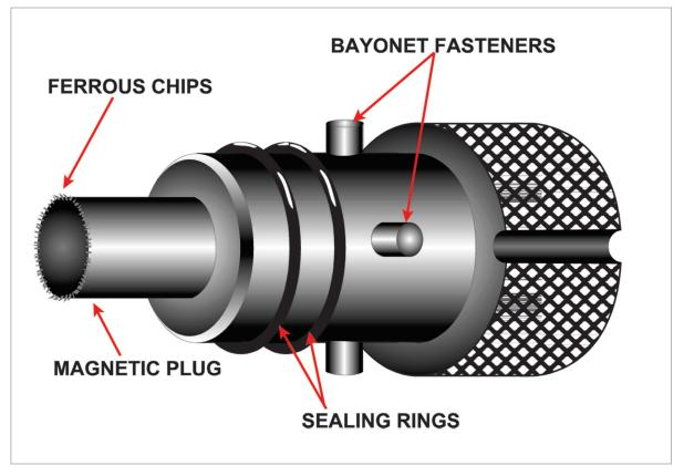
Figure 19.7 A magnetic chip detector.
