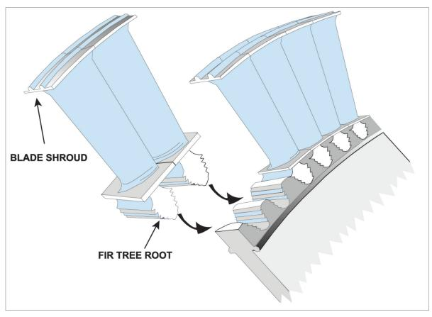
Figure 17.7 Fir tree root turbine blade attachment.
