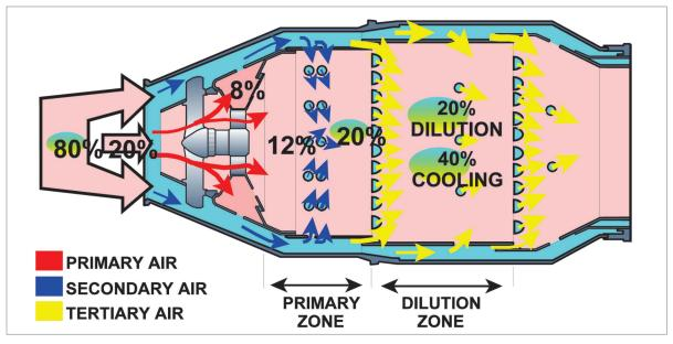
Figure 16.1 The division of airflow through the combustion chamber.
