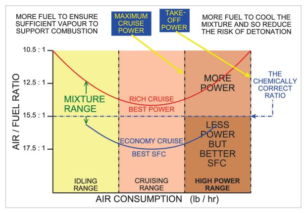
Figure 7.1 A typical air/fuel mixture curve.
