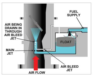
Figure 8.5 The air bleed diffuser.
