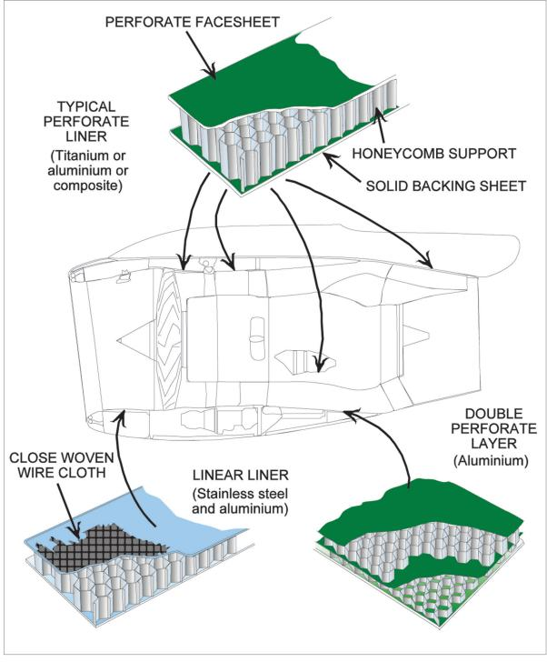
Figure 18.8 The types of materials used for noise suppression & their locations.
