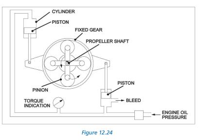
pressure of the torque transmission system. This pressure is then read off on the torque meter gauge. *Figure 12.24* shows the ring gear system.
