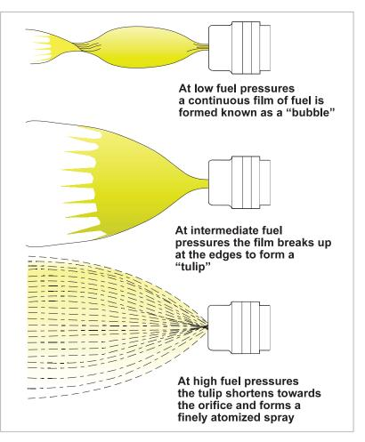
Figure 16.10 Fuel spray patterns at various pressures.
