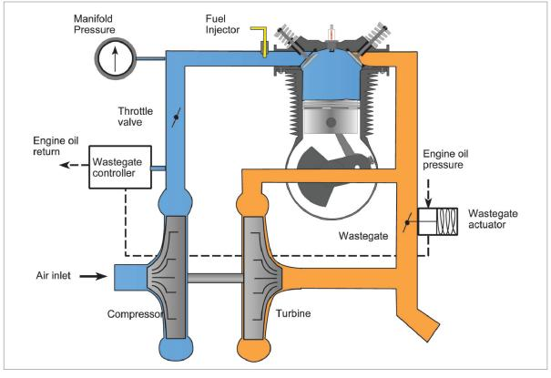
Figure 11.3 Turbocharger - general arrangement.
