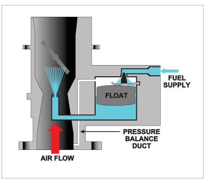
Figure 8.3 The pressure balance duct.
