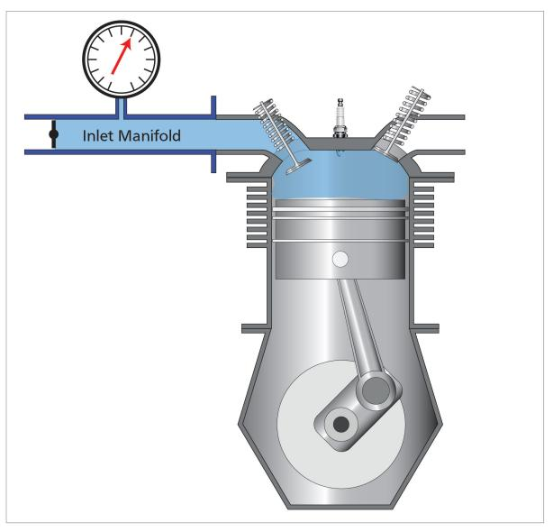
Figure 2.8 Manifold absolute pressure gauge
