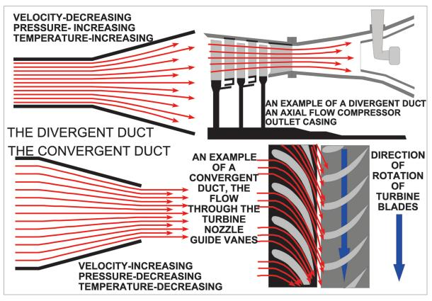
Figure 13.6 The use of divergent & convergent ducts to control the passage of airflow through the engine.
