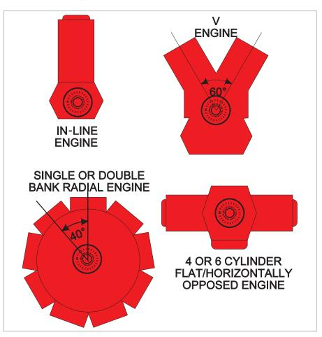
Figure 2.1 Engine Layouts
