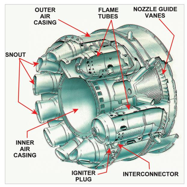
Figure 16.4 A tubo-annular combustion chamber system.
