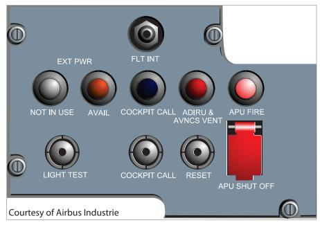
Figure 24.3 External APU control panel
