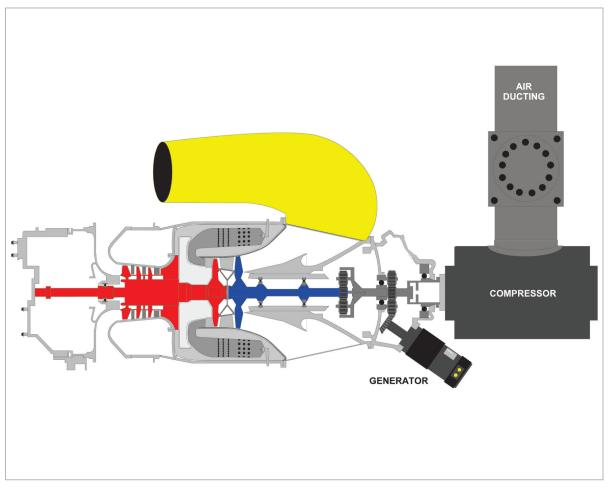
Figure 24.1 Free turbine turboshaft APU
