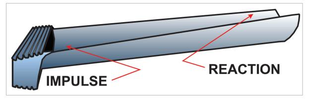
Figure 17.4 The combination impulse-reaction blade.
