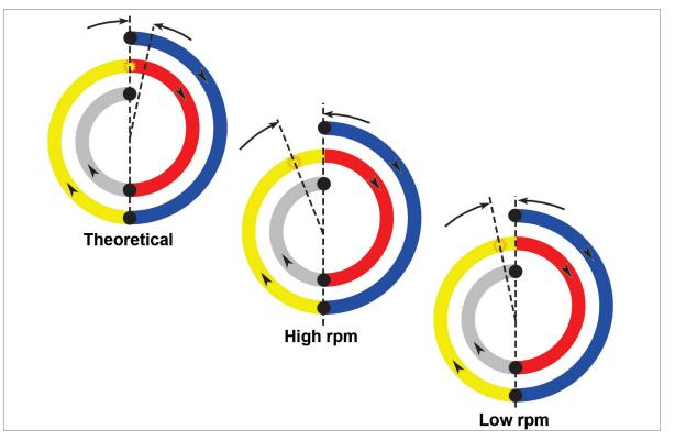
Figure 6.2 Moving the ignition point to the optimum position for idling rpm & high speed running.
