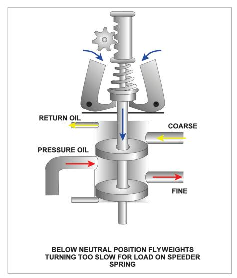
Figure 12.14 Underspeed condition.
