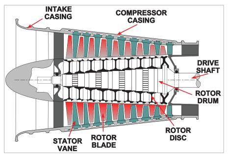
Figure 15.3 A single spool compressor.
