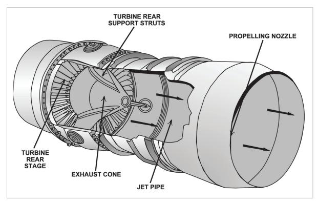
Figure 18.1 A basic jet pipe.
