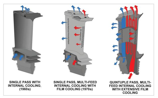
Figure 27.2 The development of turbine blade cooling
