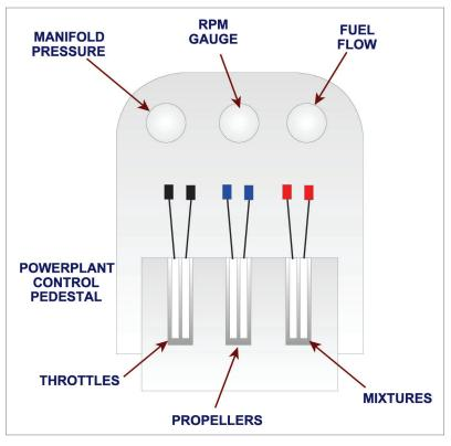
Figure 12.25 A typical light twin powerplant controls arrangement
