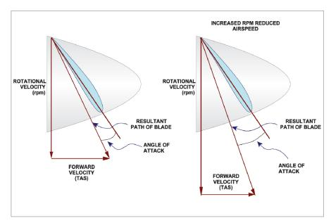
Figure 12.6 Reduced TAS and increased rpm
