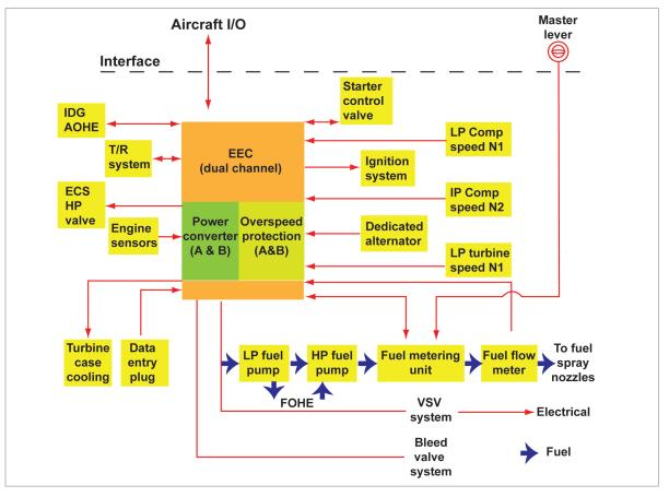
Figure 26.6 A typical FADEC structure
