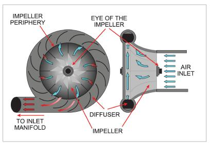
Figure 11.1 A centrifugal compressor.
